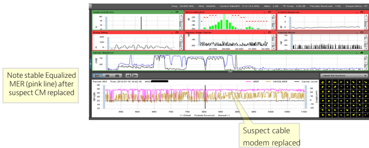
Figure 4. Equalized MER improved after replacing modem
