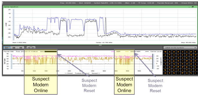
Figure 3. Improvement after resetting the modem
