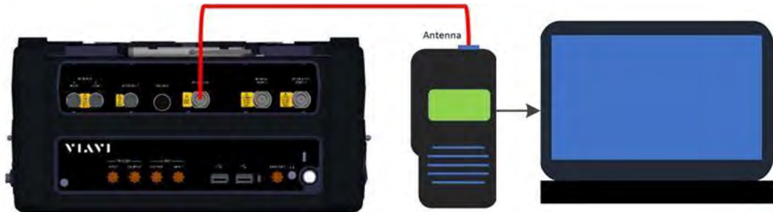
Figure 3-2 TETRA Receiver Sensitivity Test Setup Diagram
