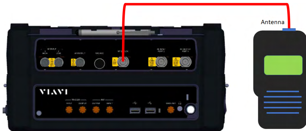
Figure 3-1 TETRA Transceiver Test Setup Diagram
